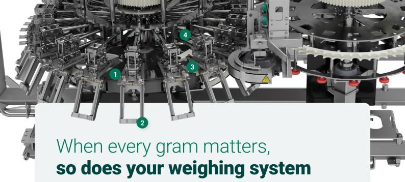
In the middle shaft, mechanically locking leg carriers 1 with integrated back support 2 keep each bird fully stable during weighing. The carriers spread eccentrically for complete bird separation and pass alternately over fixed double load cells, 3 maximizing weighing time. The robust, fixed weighing units 4 and durable mechanical design ensure long-term reliability while delivering highly consistent and precise measurements.
